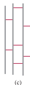
Figure 16.15 Rubber molecules ordinarily are bent and convoluted. Parts (a) and (b) represent the long chains before and after vulcanization, respectively; (c) shows the alignment of molecules when stretched. Without vulcanization these molecules would slip past one another, and rubber would lose its elastic properties.
