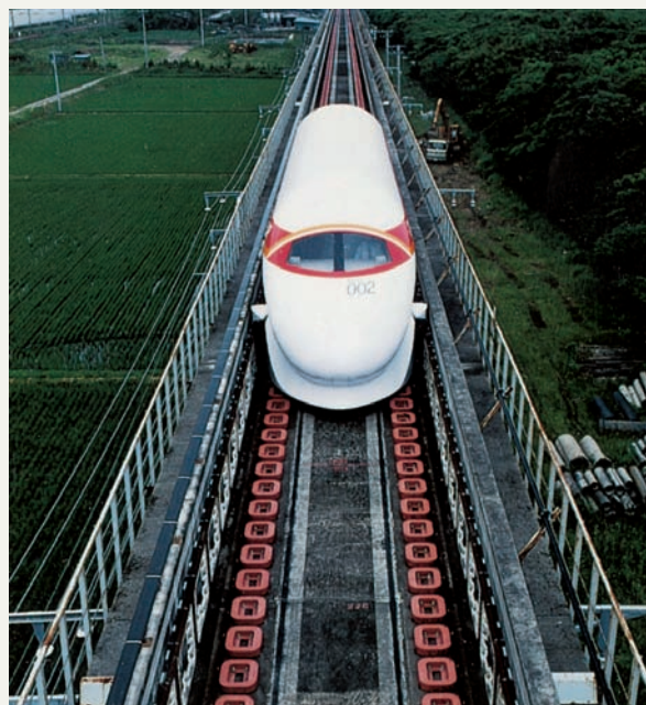
An experimental levitation train that operates on superconducting material at the temperature of liquid helium.
