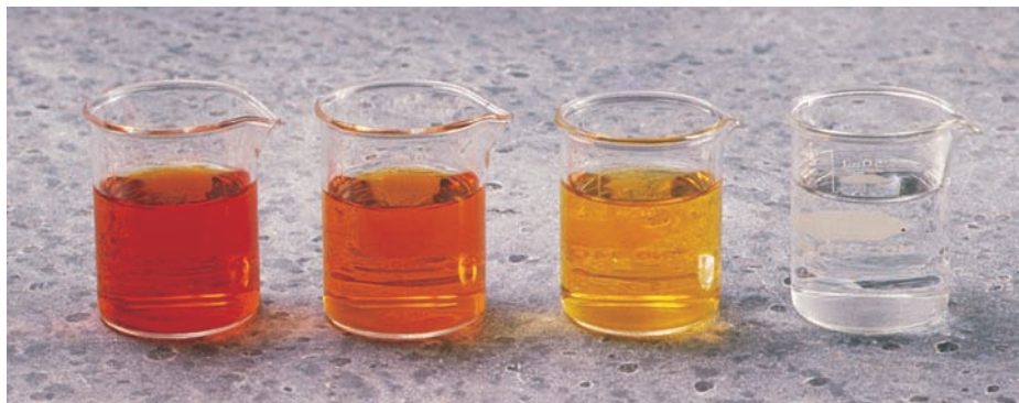
Figure 14.3 The decrease in bromine concentration as time elapses shows up as a loss of color (from left to right).
