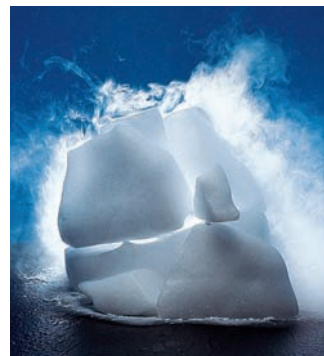
Figure 5.9 Under atmospheric conditions, solid carbon dioxide does not melt; it only sublimates. The cold carbon dioxide gas causes nearby water vapor to condense and form a fog.
