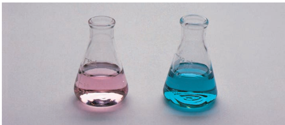
Figure 12.13 Left: An aqueous cobalt(II) chloride solution. The pink color is due to the presence of \text{Co}(\text{H}_2\text{O})_6^{2+} ions. Right: After the addition of HCl solution, the solution turns blue because of the formation of the complex ion \text{CoCl}_4^{2-} .
