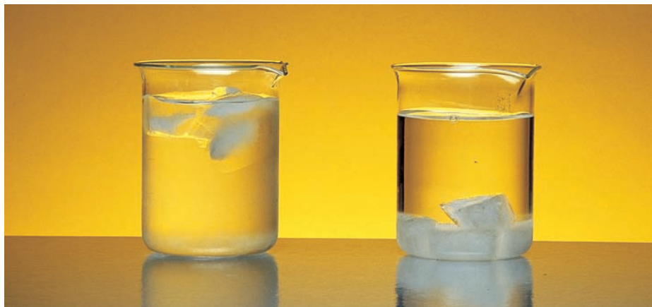
Figure 6.8 Left: Ice cubes float on water. Right: Solid benzene sinks to the bottom of liquid benzene.
