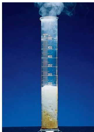
Figure 14.20 The decomposition of hydrogen peroxide is catalyzed by iodide ions. A few drops of liquid soap have been added to the solution to dramatize the evolution of oxygen gas. (Some of the iodide ions are oxidized to molecular iodine, which then reacts with iodide ions to form the brown triiodide ion \text{I}_3^- .)
