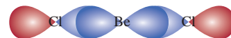
Figure 4.7 The linear geometry of \text{BeCl}_2 can be explained by assuming that Be is sp hybridized. In the valence bond model, the two sp hybrid orbitals overlap with the two chlorine 3p orbitals to form two covalent bonds.
