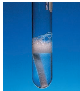
Figure 11.1 A piece of blackboard chalk, which is mostly CaCO_3 , reacts with hydrochloric acid.
