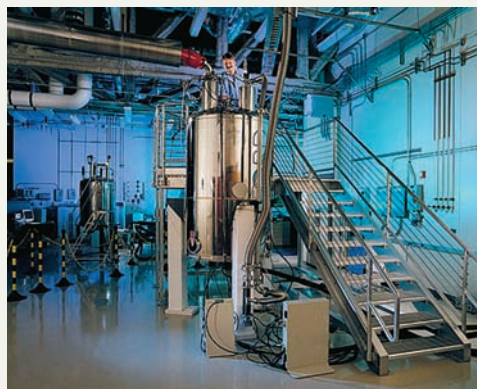
An NMR spectrometer. The instrument is surrounded by a insulated container of liquid nitrogen, which is used to cool the large electromagnets required to generate the magnetic field.
