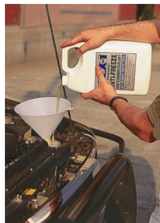
In cold climate regions, antifreeze must be used in car radiators in winter.
