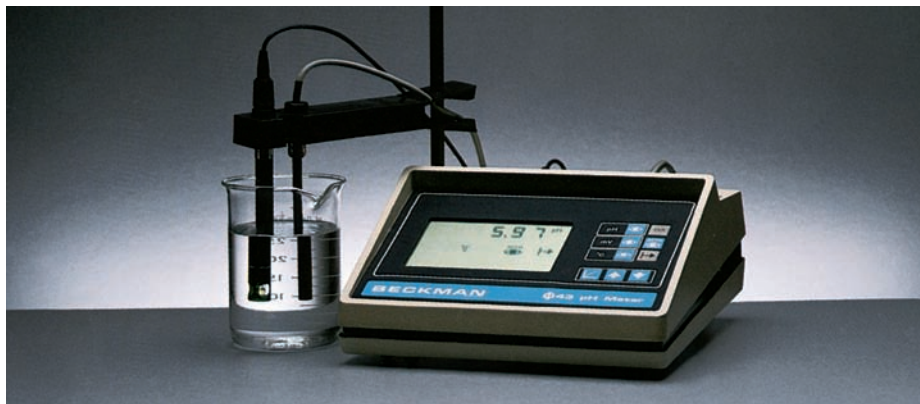
Figure 11.6 A pH meter is commonly used in the laboratory to determine the pH of a solution. Although many pH meters have scales marked with values from 1 to 14, pH values can, in fact, be less than 1 and greater than 14. The science behind the pH meter will be discussed in Chapter 13.
