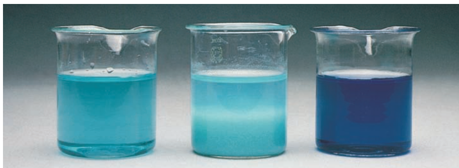
Figure 12.14 Left: An aqueous solution of copper(II) sulfate. Center: After the addition of a few drops of a concentrated aqueous ammonia solution, a light-blue precipitate of \text{Cu}(\text{OH})_2 is formed. Right: When more concentrated aqueous ammonia solution is added, the \text{Cu}(\text{OH})_2 precipitate dissolves to form the dark-blue complex ion \text{Cu}(\text{NH}_3)_4^{2+} .
