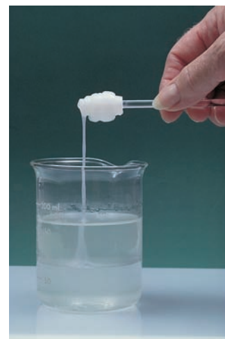
Figure 16.17 The nylon rope trick. Adding a solution of adipoyl chloride (an adipic acid derivative in which the OH groups have been replaced by Cl groups) in cyclohexane to an aqueous solution of hexamethylenediamine causes nylon to form at the interface of the two solutions, which do not mix. It can then be drawn off.
