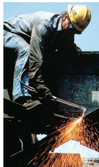
An oxyacetylene torch has a high flame temperature ( 3000^{\circ}\text{C} ) and is used to weld metals.
