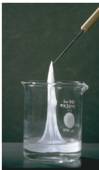
▲ Nylon is pulled from a beaker of adipoyl chloride and 1,6-hexanediamine.
