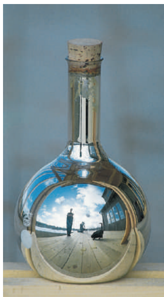
A silvered mirror has been deposited in the inside of this flask by the reaction of an aldehyde with Tollens' reagent.
